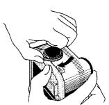
Be sure the O-ring is coated with Silicone grease all around. If opening and closing of the cover become difficult, lubricate the O-ring with the Silicone grease included in the box.
